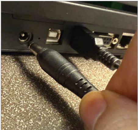
6. Connect power supply cord to printer; connect cord to SP NOTE: Use a Surge Protector and NOT a power strip (NOT supplied). An SP will help protect your printer from power surges and program failures.
