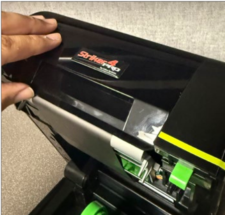
3. Clamp down ink ribbon access as shown
