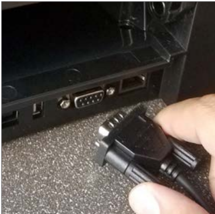
5. Connect the Striker Keypad to the printer
