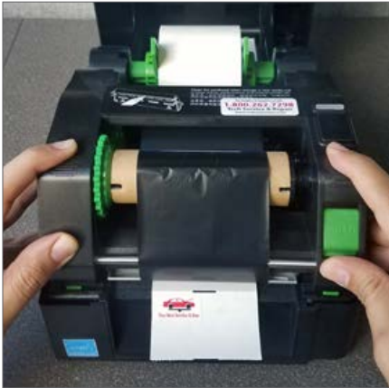
3. Clamp down ink carriage as shown
